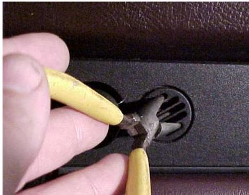
7. Remove the single Phillips head screw behind the temperature sensor vent cover.
