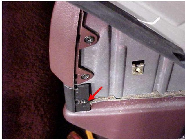
4. Carefully remove the rectangular trim cover next to the passenger side vent control lever using a small flat tip screwdriver.
