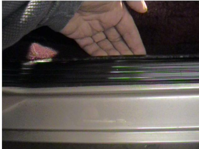
2. Pull the rubber trim off of the back of the door jamb from the bottom of the door to about 3/4 of the way up the door opening.
