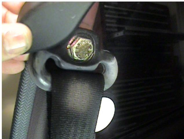
6. If your car is NOT equipped with rear shoulder harnesses, it will have a large Phillips Head screw in place of the shoulder harness mount. Remove this screw (1). Also, remove the small Phillips Head screw below and toward the rear of the car (2) from the shoulder harness mounting point.
