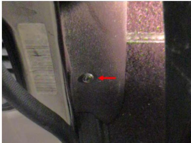
4. Remove the Phillips Head screw at the base of the trim panel below speaker opening.
