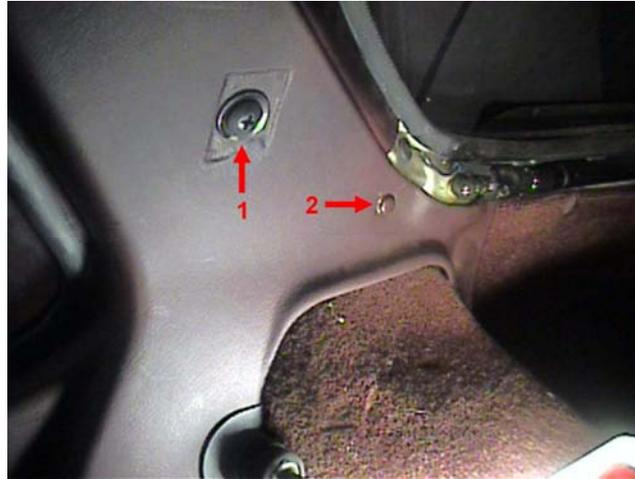
7. Remove the rubber cover from the rear seat latch pin. When you remove the cover, you'll see a hex shaped portion of the pin. Use an open end wrench to remove the latch pin.
