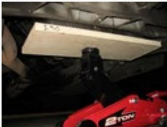
10. Use a sharp object to scribe a mark around the cross-member mounting bolts (4 per side).
