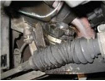
15. Before you install the new mounts, you may want to chase the threads in the mounting bolt holes of the new motor mounts with an M8 tap (i.e. retap the holes). In recent years there have been instances with OE mounts where the threads in the mounting bolt holes were not cut deep enough. This causes the threads in the holes to strip during mounting bolt installation.
