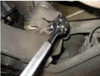
7. Remove the lower motor mount lock nuts. (M6 bolt, 17 mm open end wrench)
