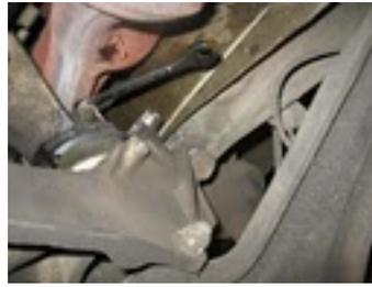
9. Place a block of wood on the pad for the floor jack (to provide a cushion). Jack up the engine on the oil pan to remove the tension on the motor mounts.
