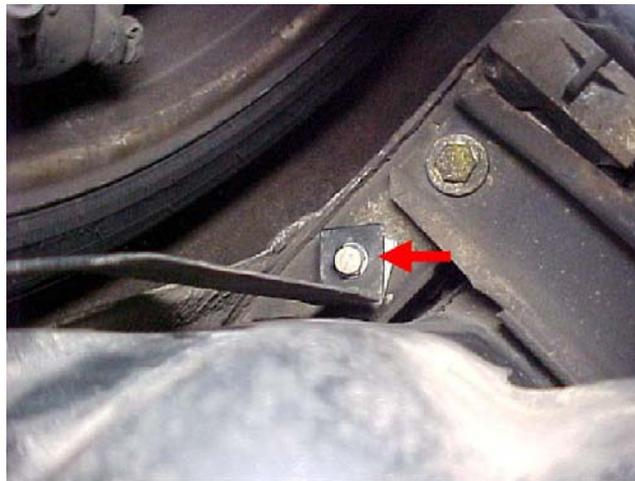
5. Locate the fuel line going from the bottom of the fuel tank to the suction of the fuel pump and pinch the rubber fuel line using a hose clamp (as shown below).
