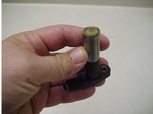
5. Install the sensor with mounted washer and tighten.
